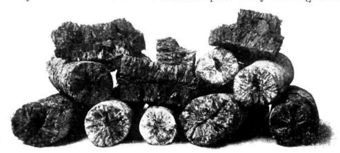
The appearance of these rods is shown in the cut where A represents a transverse section of an unused rod, and the remainder represent transverse and longitudinal sections of used rods.
